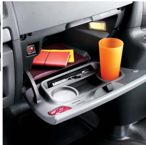
A refrigerated storage compartment is an option available with climate control.
