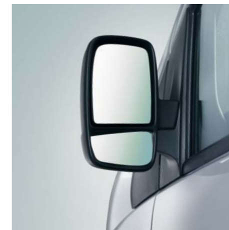
Wing mirrors feature a double parabola, giving optimum visibility and control. As an option, electric folding mirrors can be fitted. (Panorama version has single parabola wing mirrors.)
