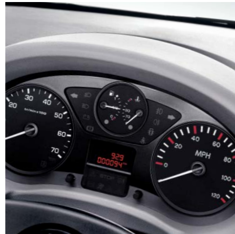
A four-dial instrument cluster features graphics on a black background for ultimate legibility.
